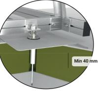
Minimum distance between Carriage Profiles and the roof surface
