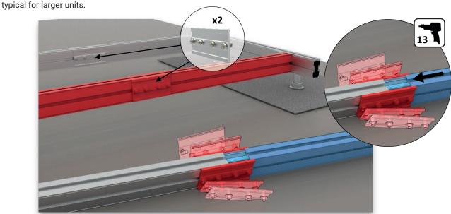
Before the Carriage Profiles can be assembled with the mounted structure the profiles must be assembled by mounting 2 pieces of the Assembly Bracket to each of the two joints.
