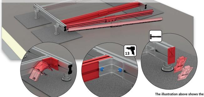
The Carriage Profile is fixed to the Installed Internal Corners by constraining the Hammer-head bolt while assuring that the position mark is oriented correctly. The final fixation is to apply the missing two Internal Corners 1 piece per profile end.
