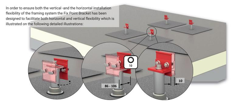
The Fix Point Bracket can be rotated and horizontally offset until the right height and position is reached.
