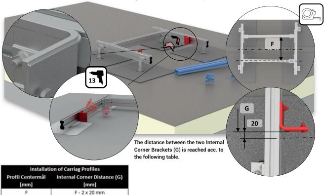
The installation of the Carriage Profiles is done on to the Cross Beam Profiles by applying 4 Internal Corner Brackets per Cross Beam. The Internal Corner Bracket does as the Fix Point Bracket and Assembly Bracket include the reinforcement rips which must be aligned with the corresponding tracks in the Carriage Profile. The following illustrations show the requirments for instaling the Internal Corner Bracket as well as the Carriage Profiles.
