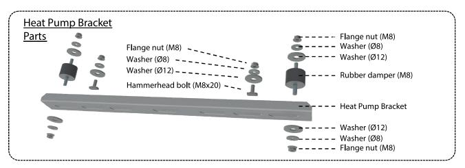
The two Heat Pump Brackets must be positioned with center distance which corresonds to the dimension (D) defined in the installation Step 6.
