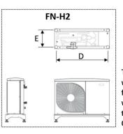
The illustration present the dimensions which can be found in the data sheet from the equipment manufacturer and where the dimension (E) is relevant for the positioning of the Intermediate Carriage Profiles.
