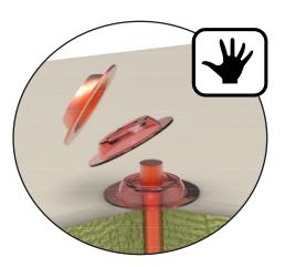
At this point the Nut and the Distance Washer is removed and the anchor is now ready for the following installation of the Roof Console
