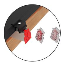
At the end of a panel row, the end cover is mounted inside the profiles so that they are shut and so that there is a reasonable visual finish to the installation.
